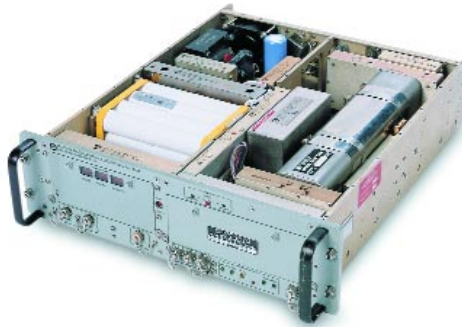
Replacement Cesium Beam Tube installation in FEI instrument
